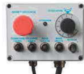
Electrical Control Control of all machine functions from the tractor cab; it can be used to adjust the rate per hectare.
