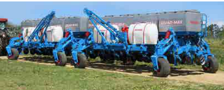
2 section QUAD-MAX type A in transport position
