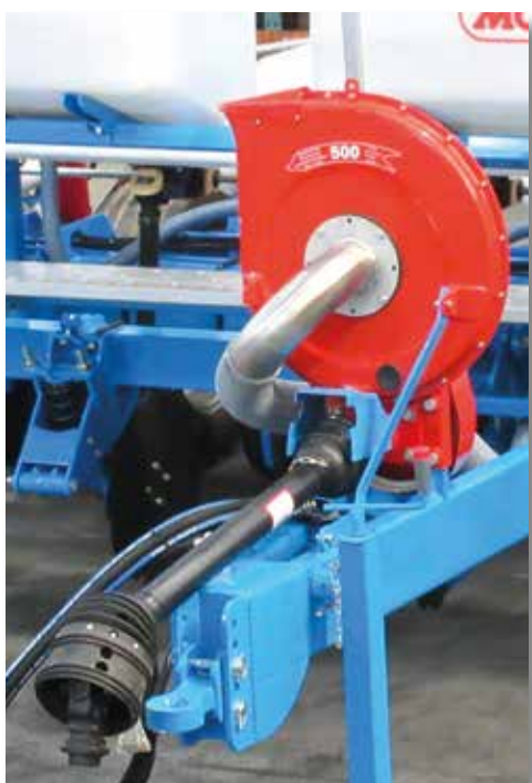
Standard drawbar with long wide-angle PTO shaft
