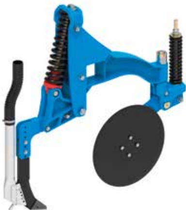
NO-TILL COULTER & TINE COMBO for hard soils
