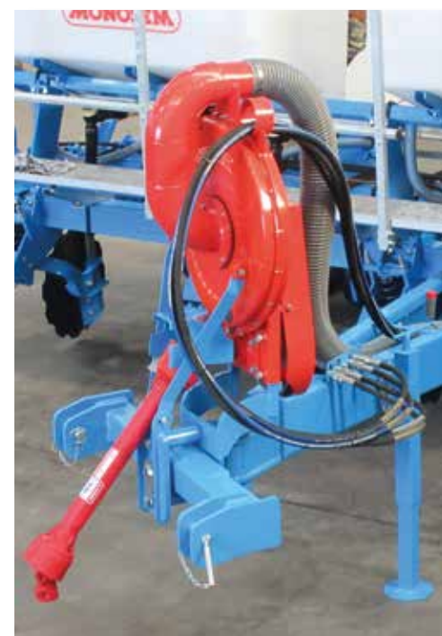
Drawbar for mounting to lift arms & short PTO shaft
